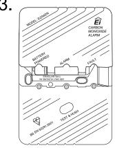
Slide the battery compartment cover off and remove.
