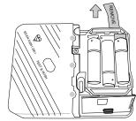
Remove the battery tab by pulling out and away from the unit.
