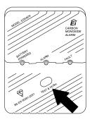
Press and hold the test button. The alarm will sound and a signal will be sent to the Pager or SignWave.
